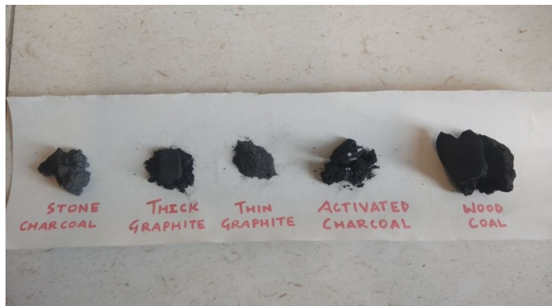
Figure 6 Different types of substances tested for making conductive paint
