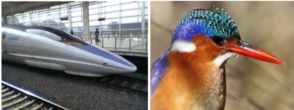
Figure 1: The streamlined design of the Japanese Shinkansen 500 Series Bullet Train (left) mimics and was modeled after the beak of a Kingfisher bird (right) to improve aerodynamics. Aircraft wing design and flight techniques are being inspired by birds and bats.
