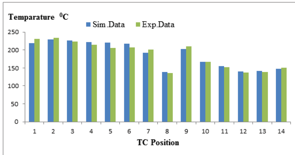
Figure 5: Simulation and experimental results of temperature distributions.
