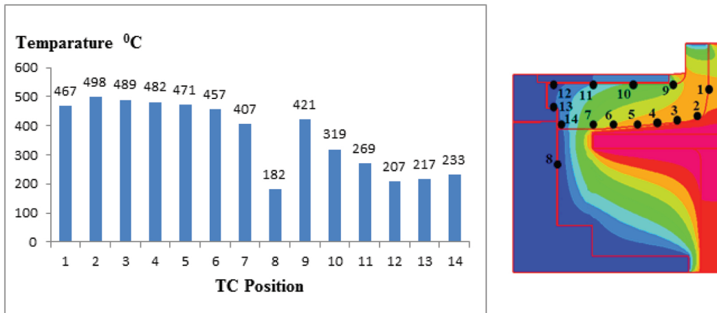
Figure 7: Simulation results of temperature distributions (Heater 600 °C, Body 180 °C).
